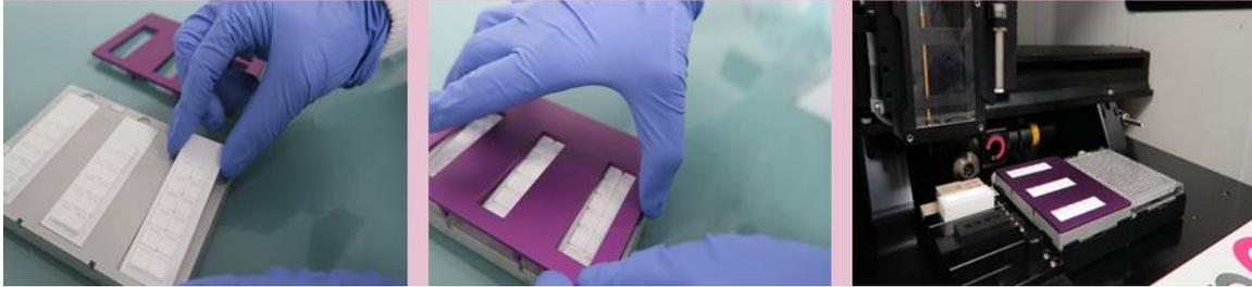
*Figure 8. proteoCHIP 12\*16 inside the cellenONE holder.*
