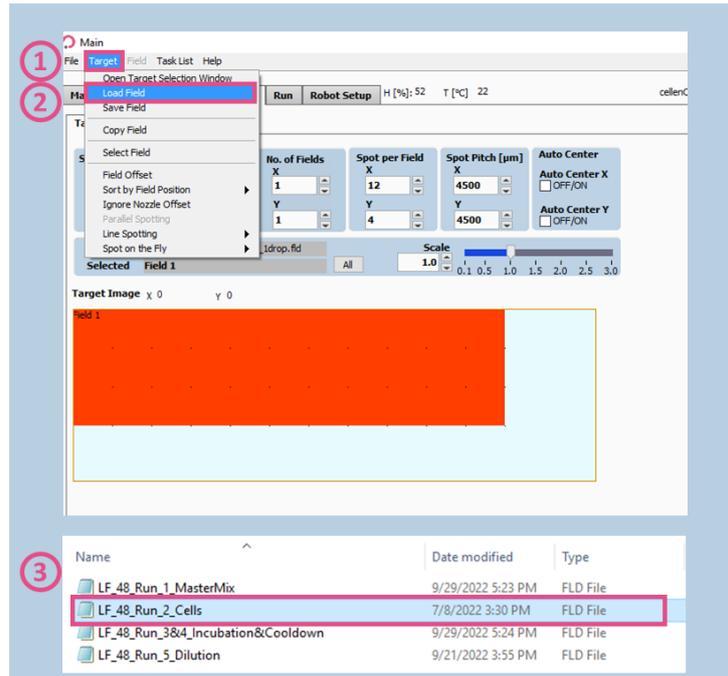
Figure 17. Load Field for cell isolation
