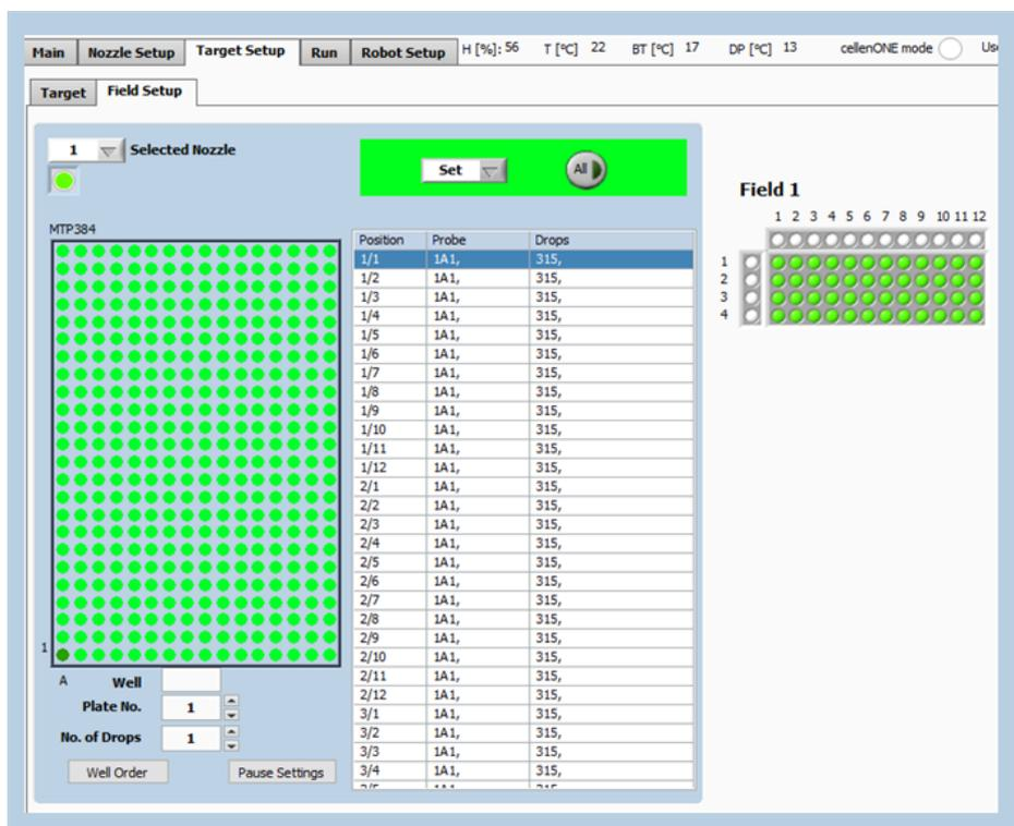
Figure 29. Field setup for incubation
