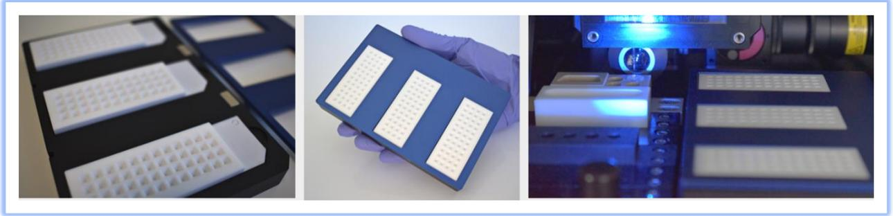
Figure 9. proteoCHIP LF inside the cellenONE holder
