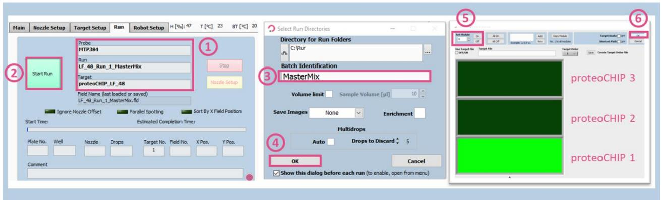
Figure 13. Starting the MasterMix dispensing run
