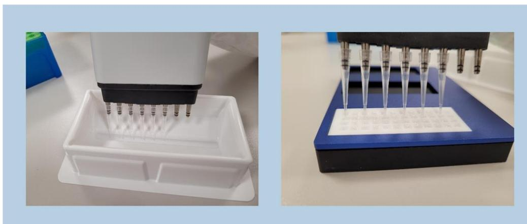
*Figure 37. Manual dilution using a multichannel pipette*
