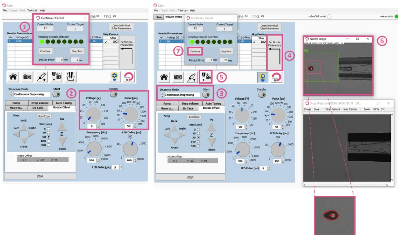
Figure 8. Drop Setup and start dispensing
