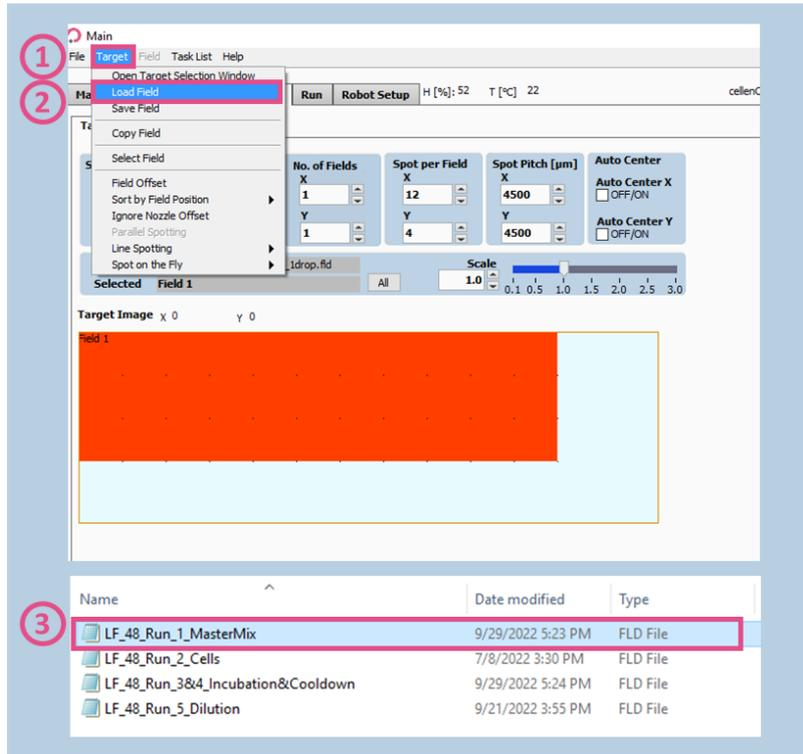
Figure 11. Load Field for MasterMix dispensing
