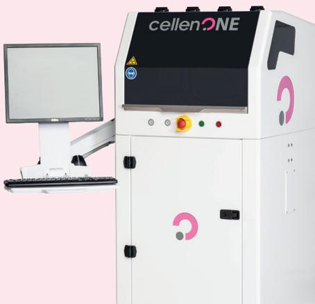
The **cellenONE®** is a unique platform combining high accuracy single cell isolation and nanoliter reagent dispensing. Image-based cell isolation ensures only single cells of interest are isolated while gentle piezoacoustic droplet generation preserves cell viability and gene expression. The same instrument also performs precision nanoliter dispensing of reagents (both aqueous and organic) allowing miniaturisation of a range of single cell omics workflows.
