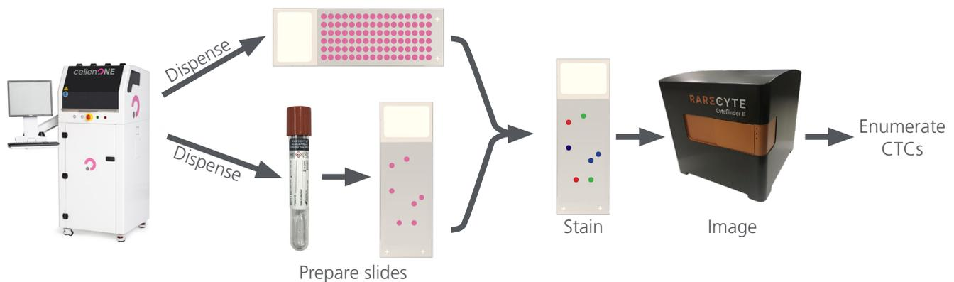
**Figure 1** 5-step CTC enumeration validation workflow. Dispense cells with cellenONE onto slides and into BCT; process BCT to slides with AccuCyte system; stain slides with RarePlex® Enumeration Panel Kit; image and analyze with CyteFinder Instrument to count CTCs.
